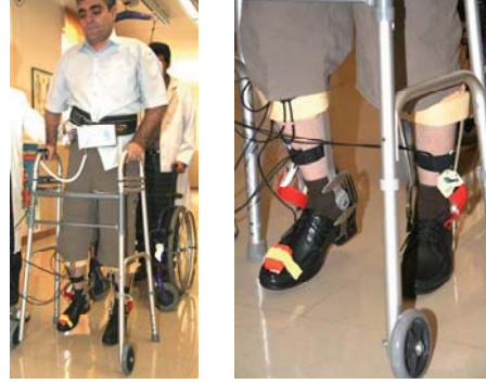
Fig. 2: A paraplegic subject with injury at T7 level uses ParaWalk to stand and walk.
